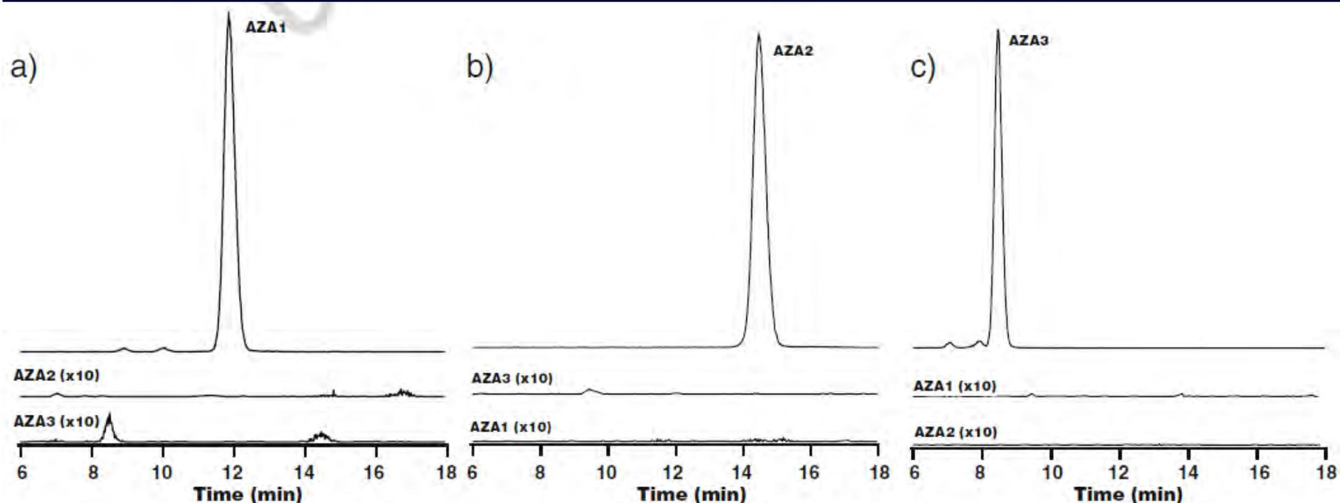
Fig. 4 LC-MS analysis of NRC CRM-AZA1 (a), -AZA2 (b) and -AZA3 (c) using MRM at  $m/z$  842.5>672.5, 856.5>672.5 and 828.5>658.5, respectively. The three MRM transitions were monitored in all three CRMs to assess potential contamination from other AZAs in the CRMs
