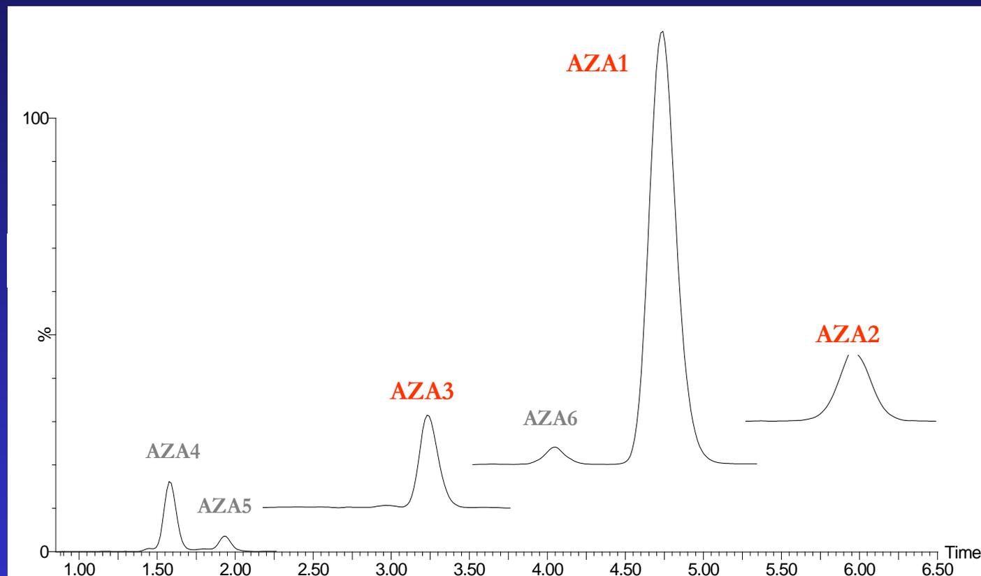
Acquired on 2795 Waters HPLC coupled to a Micromass Q-TOF Ultima (Z-spray ESI). Isocratic elution on C<sub>18</sub> ACE (30 mm x 2.1 mm) using 60 % B (Binary mobile phase with A (100 % aqueous) and B (95 % acetonitrile) each containing 2 mM ammonium formate and 50 mM formic acid).
