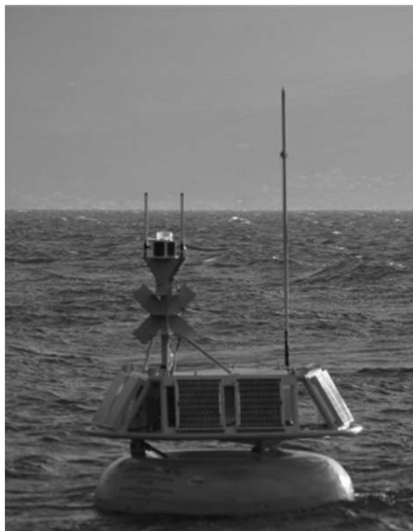
Figure 4. BOREL buoy that will transmit data between the SEAMON seabed stations and the Iridium satellite constellation.
