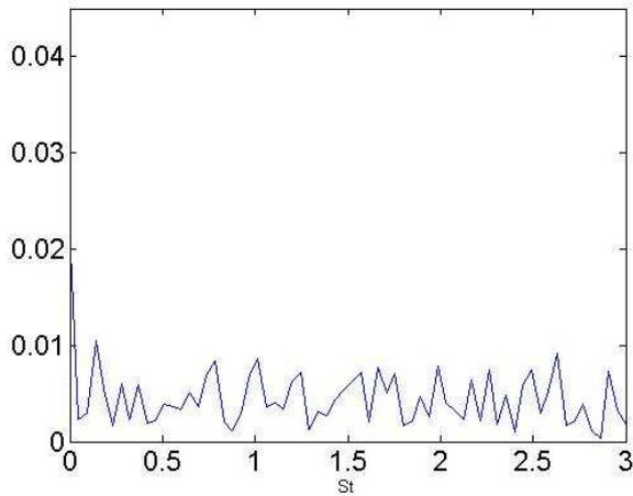
Figure 13. Power spectra computed from the  $u$  velocity component saved at  $p3$  location and projected onto (a) the whole set of available POD modes (raw original PIV database) ; (b) the first 5 POD modes; (c) from POD mode number 6 to POD mode number 20 ; (d) the residual POD modes (up to mode number 21).
