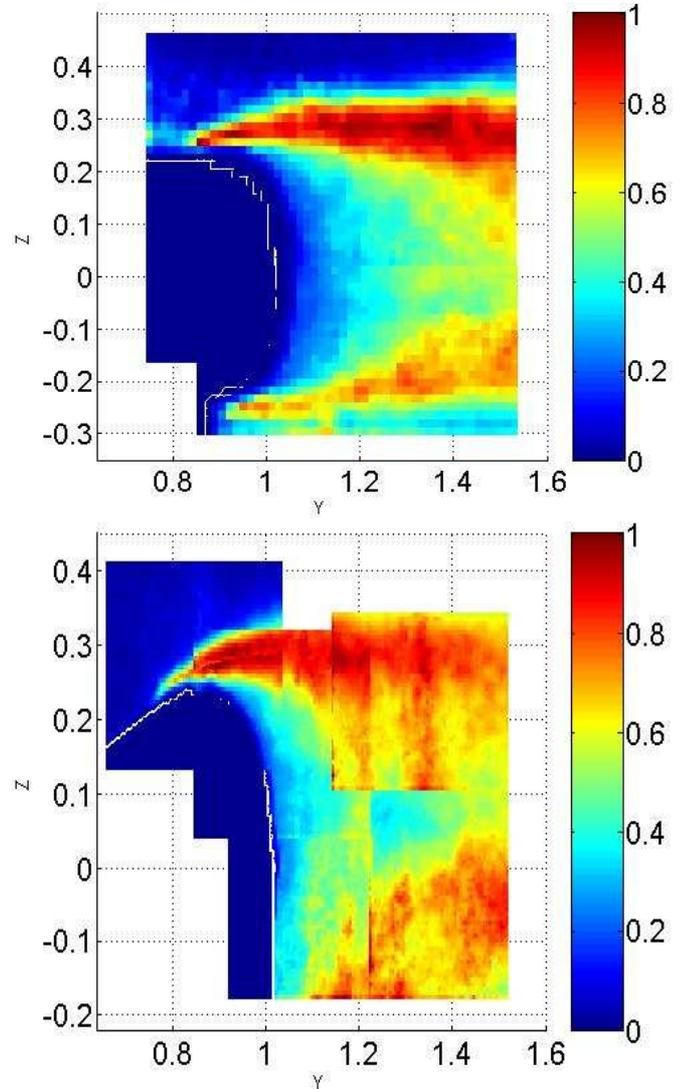
Figure 7. Normalized turbulent kinetic energy: Top: computed in each PIV plane of the first measurement campaign. Bottom: computed in each PIV plane of the second measurement campaign.
