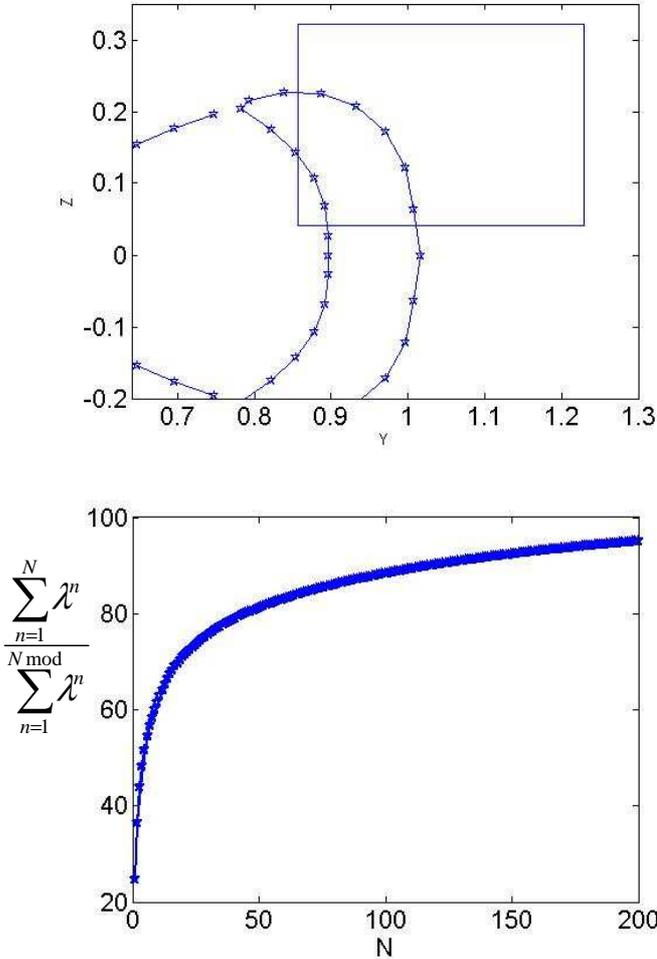
Figure 8. Top: Detailed PIV measurement plane under POD investigation. Bottom: the POD energy convergence.
