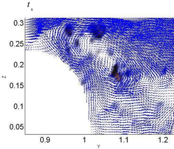
Figure 10. Successive time instantaneous vector fields projected on the first 44 pod modes which contain 80% of the total kinetic energy. Isosurfaces of Q criterion is superimposed onto each velocity vector field. Black color indicates the high positive level of Q.
