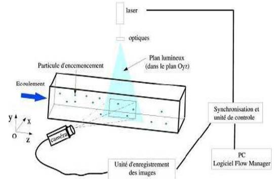
Figure 2. PIV system principle.
