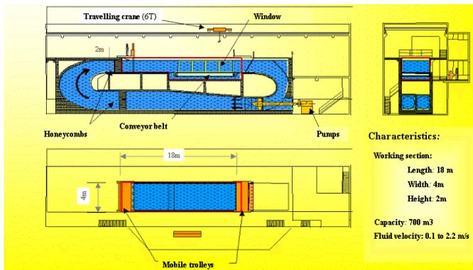
Figure 1. Ifremer free surface hydrodynamic water tunnel.
