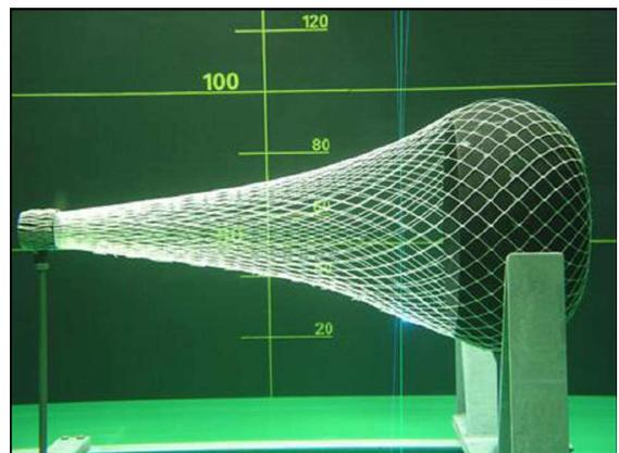
Figure 3. Rigid cod end in the flume tank.
