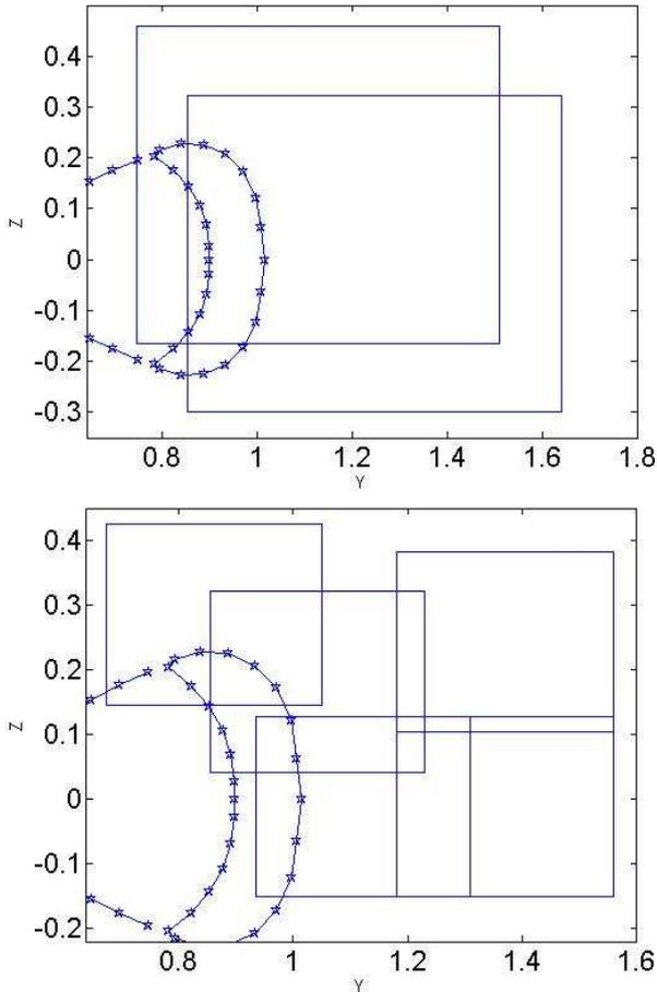
Figure 4. PIV measurement planes for the first campaign (top) and the second one (bottom).
