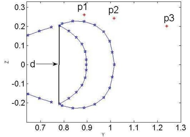
Figure 11. Detailed of the locations from which instantaneous velocity is used to compute its corresponding power spectrum. The length d is used as reference length to compute the Strouhal number.
