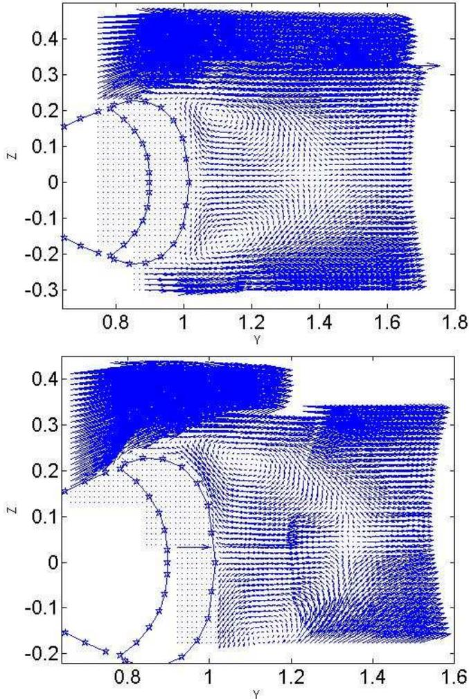
Figure 6. Mean velocity field. Top: computed in each PIV plane of the first measurement campaign. Bottom: computed in each PIV plane of the second measurement campaign.
