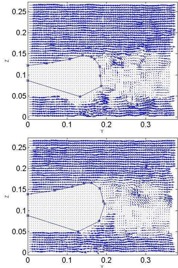
Figure 5. Instantaneous fields around the bottom trawl cod end.
