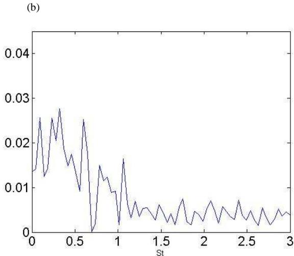
Figure 12. Spectra of the longitudinal velocity expressed as a function of Strouhal number. Top: Computed in point p1. Bottom: Computed in point p2.
