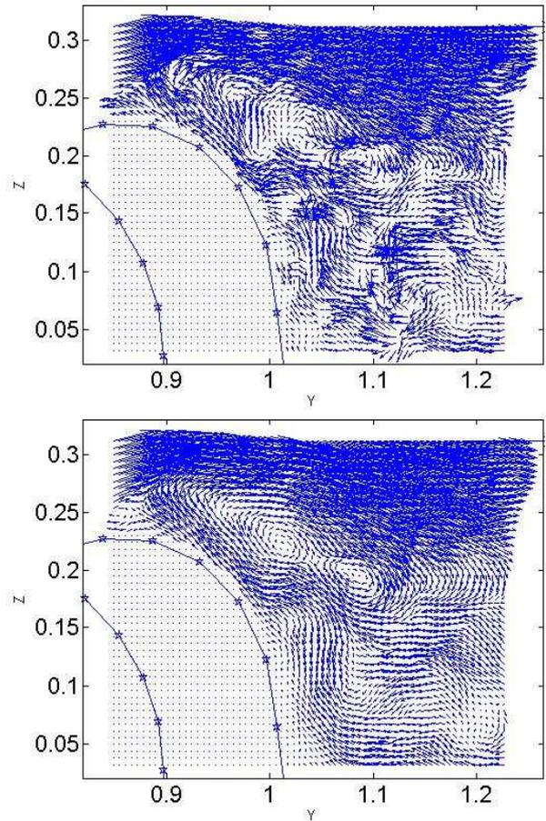
Figure 9. Top: Instantaneous PIV velocity field . Bottom same instantaneous PIV velocity field projected on the first 44 pod modes.
