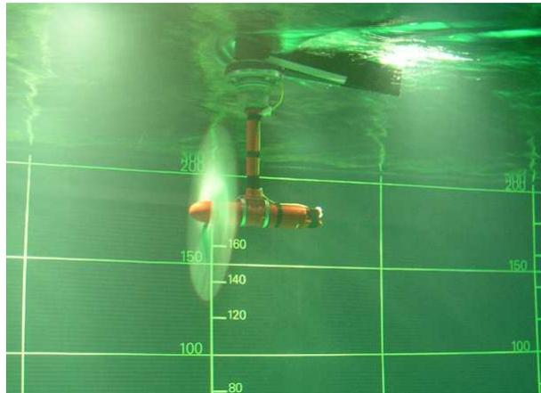
Figure 2: Fully submerged turbine now developed by TGL and model turbine during trials in the Ifremer tank
