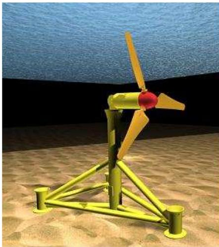
approximately 4%. The model was tested at speeds ranging from 0.5 to 1.5 m/s and the turbine performances obtained over a range of rotor speed from 10 to 190 rpm and blades pitch angle from -5 to 15 degrees. The results have been presented in [6].
