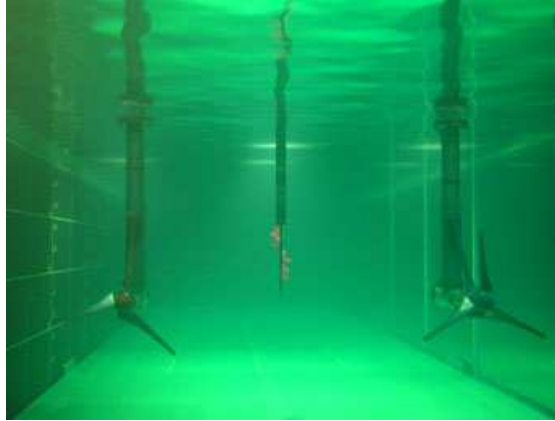
Figure 8. wake interaction effects characterization behind two turbines in close proximity
