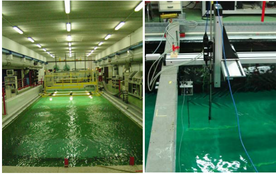
Fig 2. View downstream of the IFREMER water channel (left), installed mesh disk rig and ADV mounted on 3-dimensional axis
