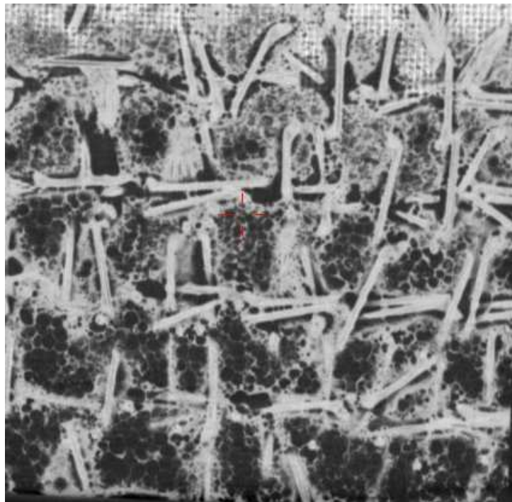
Figure 11. Adhesive layer showing folded pins at the core/skin interface plane.
