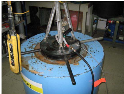
Figure 4 Pressure chamber used at Ifremer
