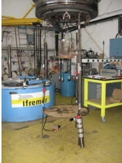
Fig. 1: Configuration of the hydrophones and velocimeter.
