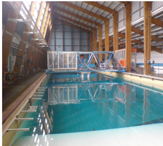
Fig. 2: Model mounted on the carriage in IFREMER Wave Tank.
