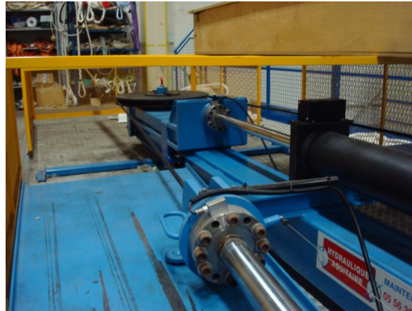
Figure 3. Bend over sheave cyclic loading of marine sling.
