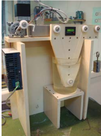
Figure 2. Yarn on yarn abrasion test.
