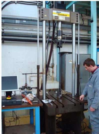
Test frame for cyclic tests
