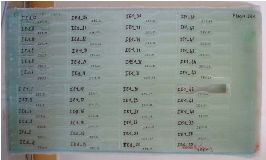
Figure 57. Infused E-glass plate IE1 after high pressure water jet cutting
