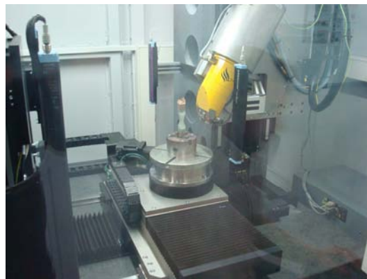
Figure 53. Four samples during analysis by tomography
