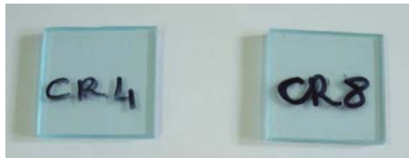
Figure 54. View of the sea water ageing specimens (pure resin at 20^{\circ}\text{C} and 40^{\circ}\text{C} )
