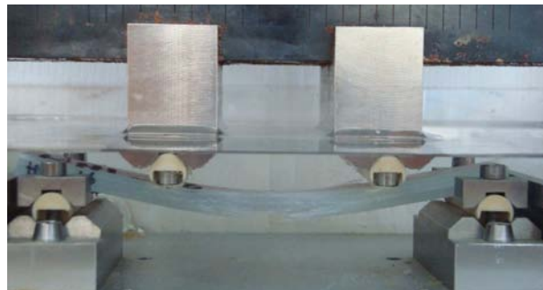
Figure 64. Fatigue test set-up in four-point bending in natural circulating sea water
