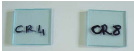
Fig. 11. View of the sea water ageing specimens (pure resin at 20°C and 40°C)
