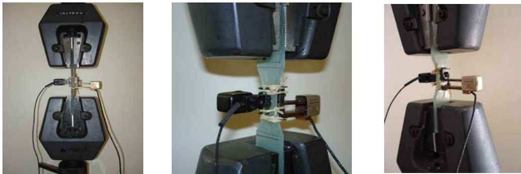
Figure 61. Load device and instrumentation of the “CRP” tensile tests
