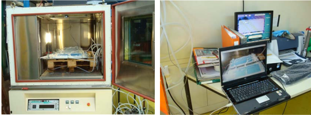
Figure 48. Infusion in the climatic chamber and visual control device
