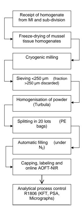
**Figure 3:** Schematic overview of process for transformation of wet mussel homogenate into CRM-FDMT1 at the IRMM.
