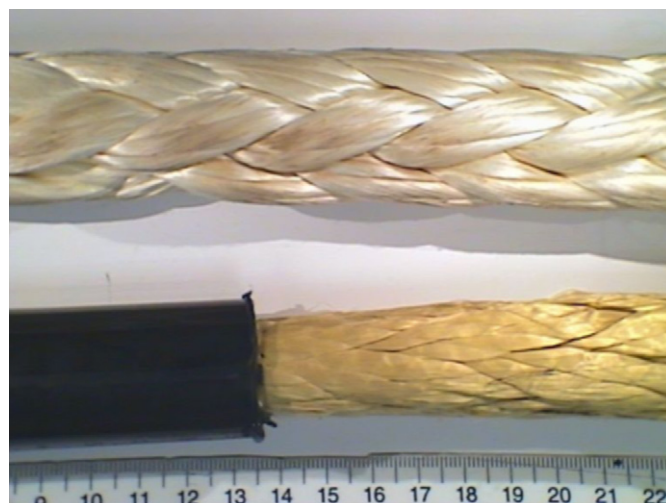
Fig. 1. Handling rope constructions, upper; HMPE, lower; coated Technora.
