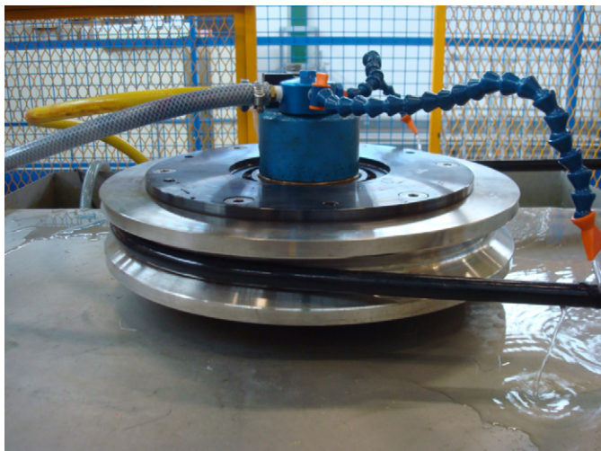
Fig. 11. Bend over sheave (BOS) test on jacketed aramid, rope wetted continuously during test.
