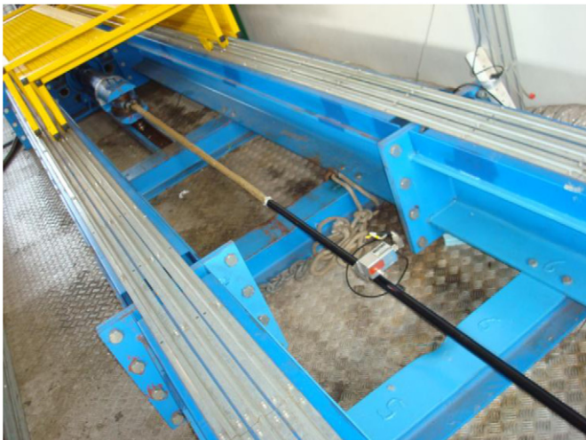
Fig. 2. Part of aramid rope on 100 ton test frame with wire transducer in place. Cover removed at rope ends for splicing.
