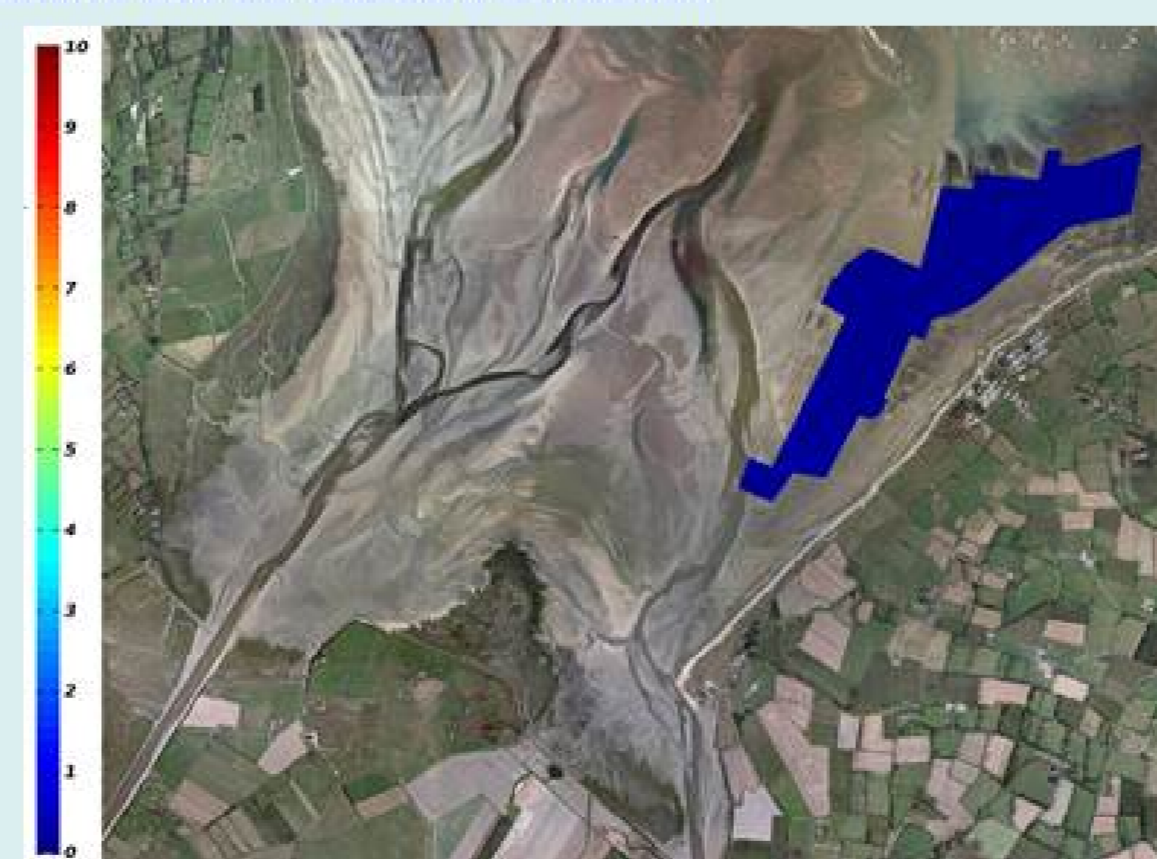
Oyster dry flesh mass differences (expressed in %) between the scenario and the standard simulation after one year
