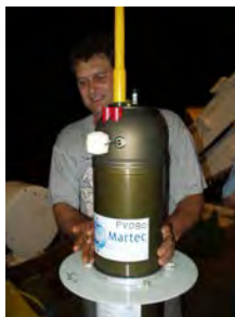
Figure 4: Profiling float PROVOR equipped with Seabird sensor (left) and FSI (right)
