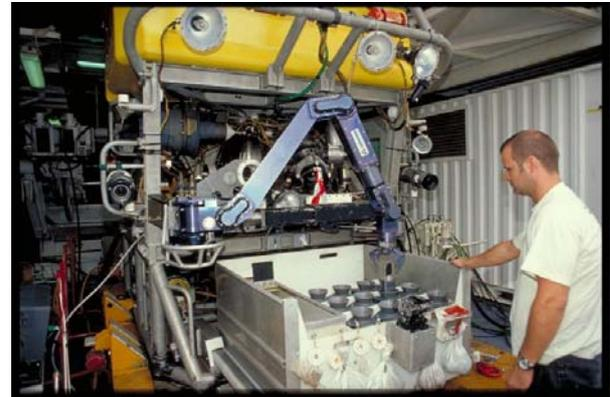
**Figure 7. The Victor 6000 ROV and its hydraulic manipulator**
