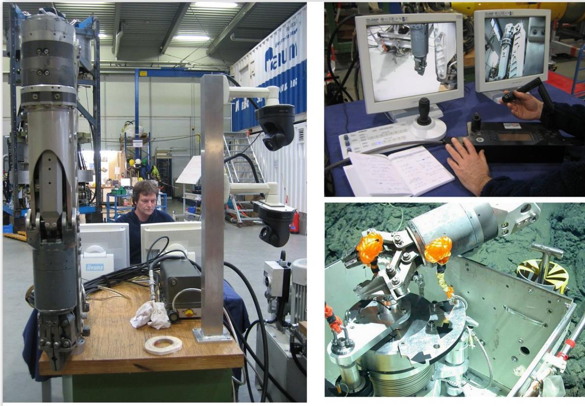
**Figure 10. Hydraulic Manipulation Training Stand at MARUM, Bremen. The easy to use setup allows regular pilot exercise, training of 3D perspective viewing with 2 adjustable 2D camera feeds, and design support or optimization of complex tools (shown is a pressure tight sampling system istalled in the sample-drawer of QUEST).**
