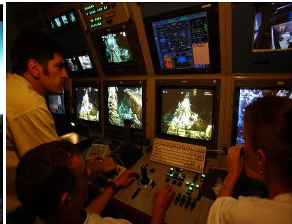
**Figure 8. Subsea tele operation phase with video feedback in the ROV control room**
