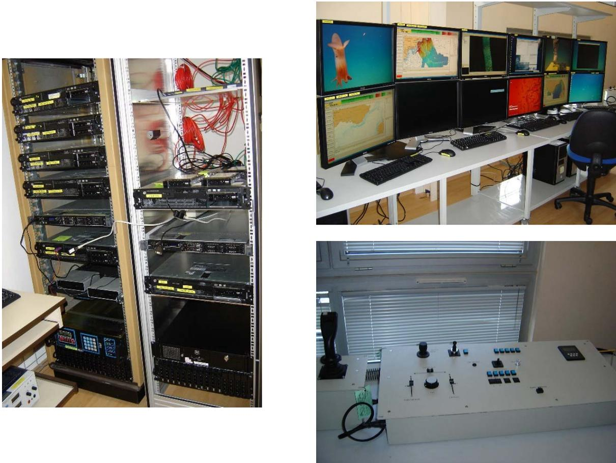
**Figure 6. Platform Implementation: PC and network switches rack (left); Operator control displays (top right); operator piloting console (bottom right)**
