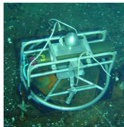
Pressure sensor deployed on the Lucky Strike lava lake (Graviluck 2006)
