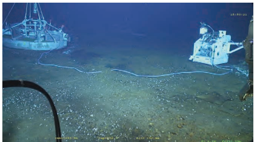
Above: the SEAMON East node was deployed at the base of the Tour Eiffel active edifice. Momarsat cruise 2010 (c) Ifremer
