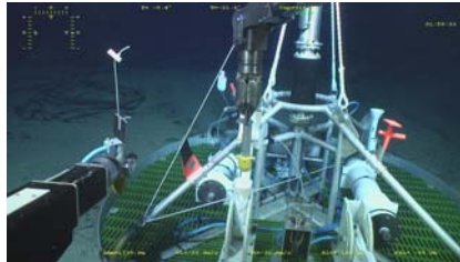
Underwater connexion of the OBS JPP module.
