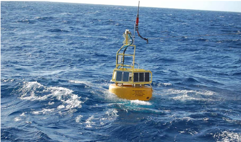
The BOREL buoy sends the data acquired on the seafloor to IFREMER-Brest via satellite. © Ifremer/Jozée Sarrazin
