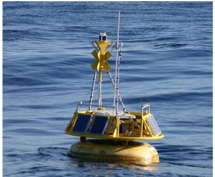
Figure 3: Borel buoy that will assure data transmission relay between the SEAMON seabed stations and the Iridium satellite constellation
