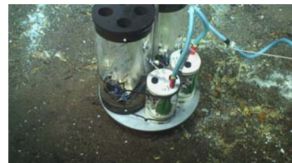
The IronMan chemical analyser deployed on small cracks.
