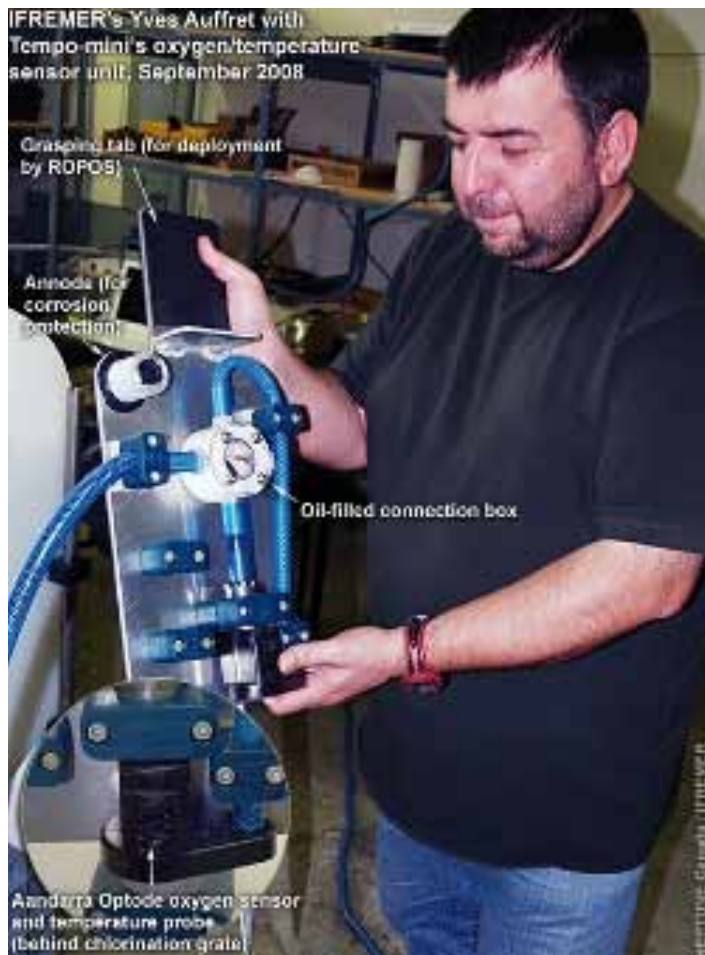
Fig.4 - IFREMER's Yves Auffret with Tempo-mini's Aanderaa optode oxygen sensor and temperature probe.
