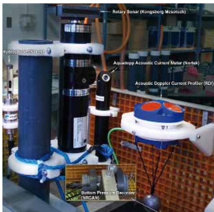
Fig.3 - Instruments installed on a platform and ready for deployment in Saanich Inlet, September 2008. From left: hydrophone, rotary sonar, current meter and ADCP. Bottom pressure recorder at base of platform.
