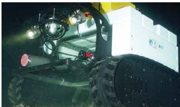
Fig.18 - Wally Hydrate Crawler in action
