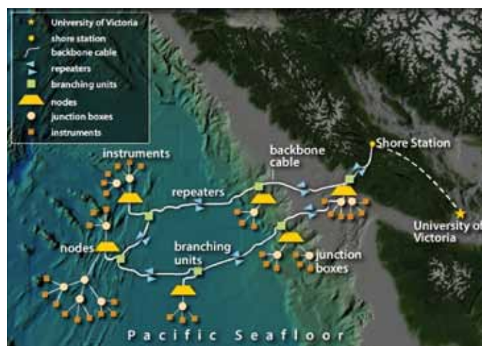
Fig.2 - Basic design of Neptune Canada infrastructure.
