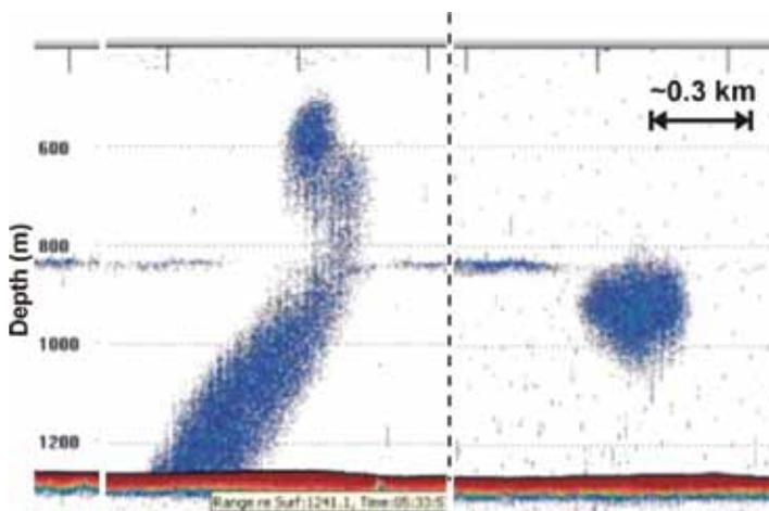
Fig.8 - Gas plumes above the HMMV in July 2005 as seen in the 18kHz fishfinder echolot. Note the bow of the plume and the floating separated plume due to the currents.
