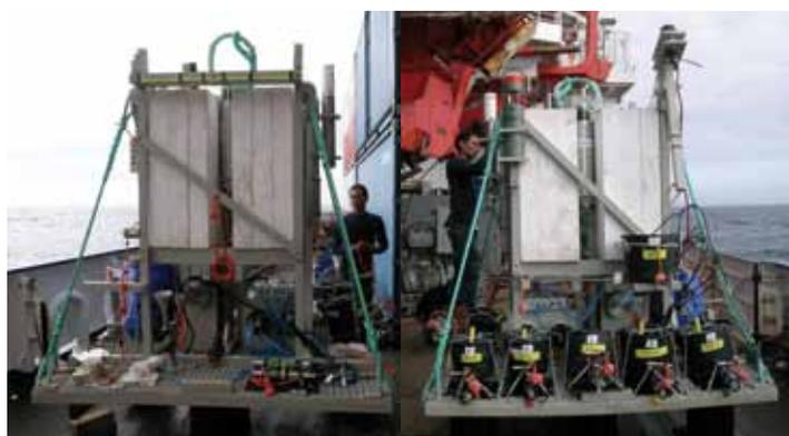
Fig. 20 - LOOME just before deployment, left panel, Backside with central data storage, CLSI (funnel) and Costof, right photo: front side with T and chemosensor strings, sonar and CTD. The white blocks are flotation material.
