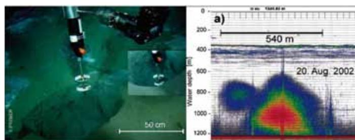
Fig.4 - Methane plume in the water column (right) and a seep seen on the seabed (left).
