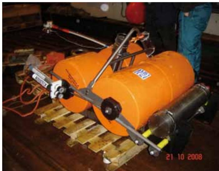
Fig.5 - The Ocean Bottom Seismometer (OBS) system (UiT including geophone, buoyancy, recorder, acoustic releaser, sender and flash light, and weight.
