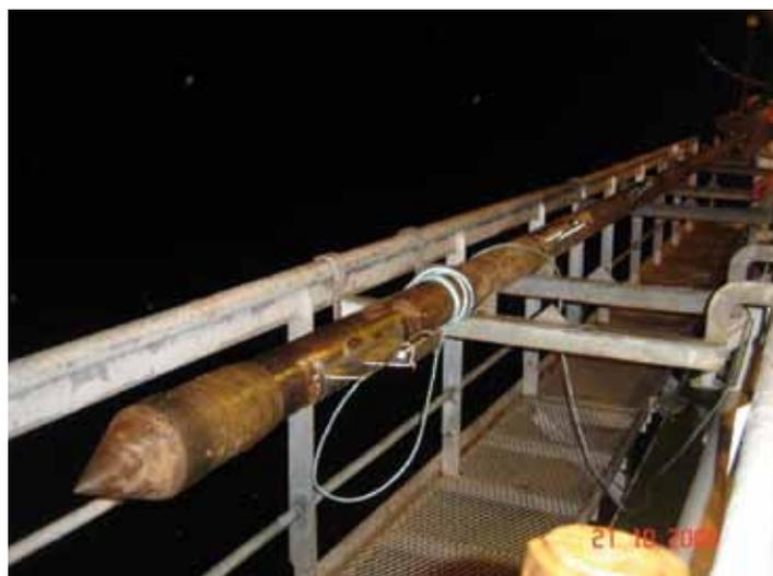
Fig.6 - T-lance equipped with thermometers mounted on outriggers along the external wall of the pipe at intervals of 1.40 m. Picture taken on-board the RV Jan Mayen prior to deployment.
