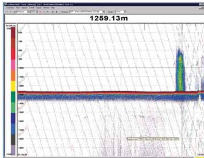
Fig.9 - Gas plume above the HMMV in October 2008 as seen in the 18kHz "plumefinder" echolot. Note that the plume has no horizontal deviations indicating weak currents during the time of the recording.
