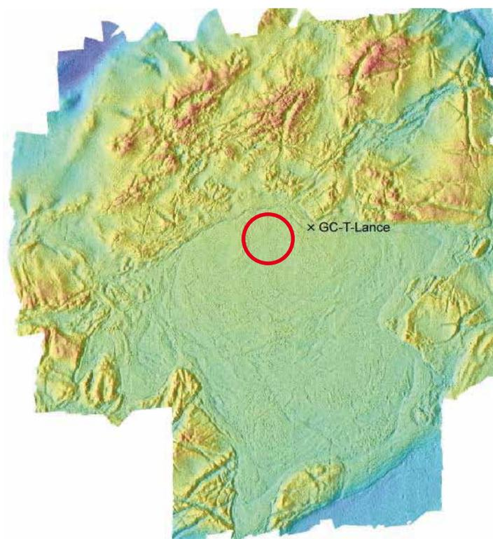
Fig. 16 - Hot spot area. Microbathymetric map from 2006 (Source IFREMER), with a 10 times higher resolution. The hot center is indicated with a red circle. The X indicates the position of the graviticorer with attached temperature probes.
