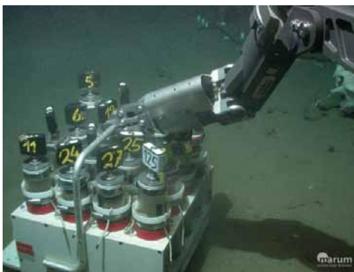
Fig.10 - The push core rack
