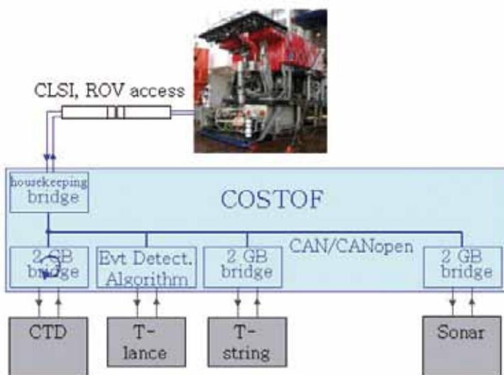
Fig. 21 - Costof implementation on the Loom observatory
