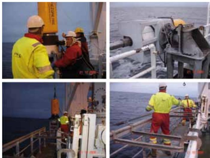
Fig.7 - Picture captions from top left to bottom right: 1. P-lance being assembled in its rotating frame prior to deployment. 2. P-lance head in its rotating frame. 3. P-lance soon to be deployed. 4. P-lance being deployed from the RV Jan Mayen.
