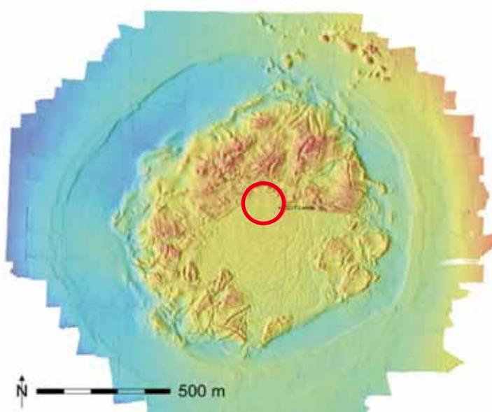
Fig.3 - Bathymetry map of the HMMV from 2003 (courtesy, J.-P. Foucher, Ifremer). The position of the previous temperature lance is indicated by a star. The three instruments of LOOME 1st part are all located in the northern part of the HMMV caldera (red circle). The volcano is surrounded by a slight depression. The hilly area is the hydrate periphery. The central area has few features
