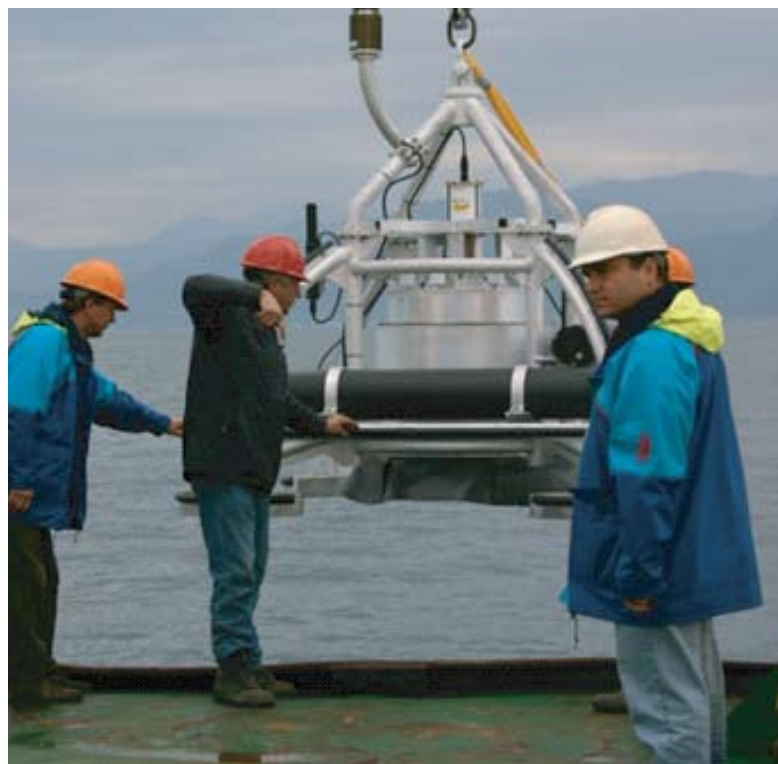
Cable deployment of ORION 4 in the ASSEM Gulf of Corinth network
