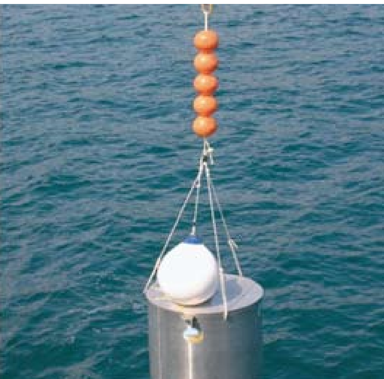
Geodetic base to be deployed with the help of a submersible
