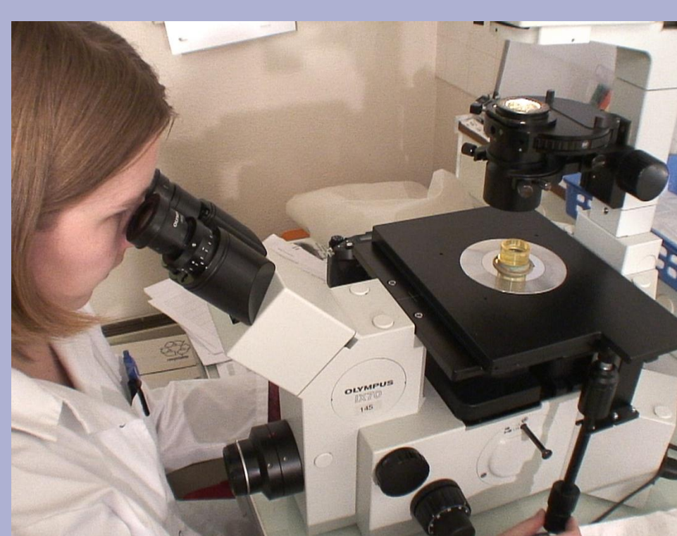
Numeric determination of the algae concentration by using reverse optical microscope
