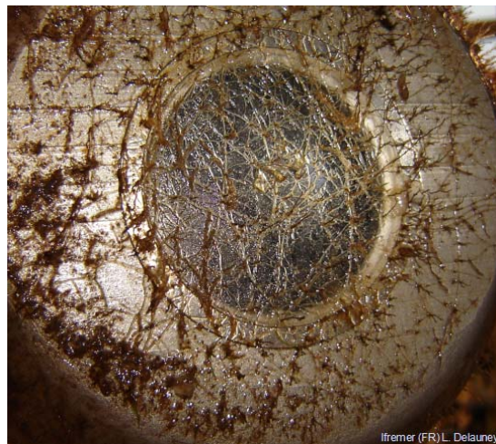
Fig 2 : Transmissometer after 40 days in Trondheim harbour (Norway) during summer
