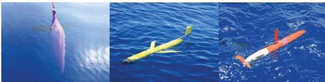
Figure 1: The three operational gliders (from left to right: Seaglider, Slocum, Spray) transferring, while at surface, the data they just collected underwater and receiving new commands thanks to the bidirectional link Iridium link.
