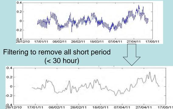
Fig. 5 Up, hourly sea level data for Station 1. Down, low pass filtered data.
