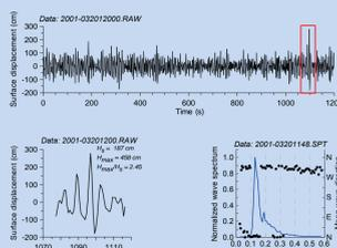
Fig. 6. Time series of the sea surface, extreme wave shapes and spectrum.
