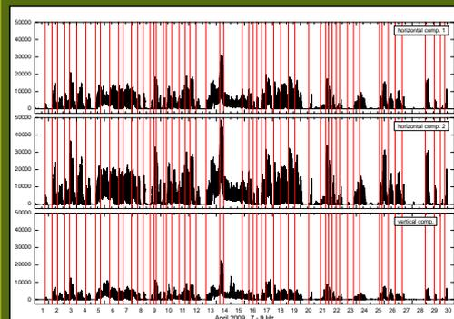
Butterworth band-pass filter was applied on the records for frequency intervals 3-5 Hz and 7-9 Hz. The envelopes of filtered records were calculated and smoothed by running average (example of filtered one-month 3 component records is shown on the left side).
