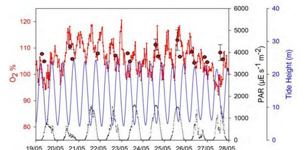
Figure 6. Variation of DO<sub>2</sub> (red line), tide height (in m, blue line) and PAR (in µE s<sup>-1</sup> m<sup>-2</sup>, black dotted line) at the buoy ASTAN and DO<sub>2</sub> (red points) for the FerryBox data extracted in the vicinity.
