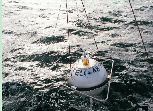
Fig. 3. Directional Waverider.
