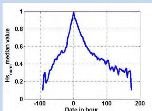
After normalizing all  $H_s$  by their maximum value  $H_{smax}$ , all swell events are superposed on the same graph.
