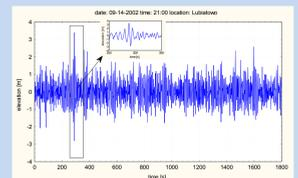
Fig. 10. Time series of the sea surface and maximum wave shape for the record from Lubiatowo.
