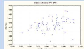
Fig. 7. Statistical skewness vs. significant wave steepness for records from Lubiatowo.
