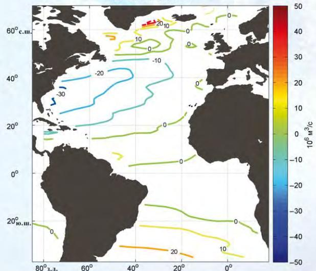
Fig.3 Example of monthly mean Sverdrup transport ( $1 \times 10^6 \text{ m}^3/\text{s} = 1 \text{ Sv}$ ) distribution the North Atlantic
