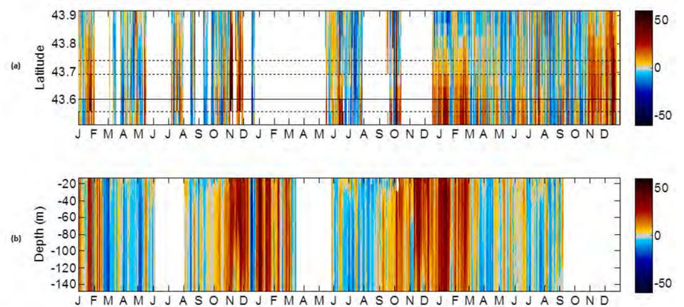
Figure 6: (a) East (positive) - west (negative) along slope currents at the HF radar nodes within the transect shown in Figure 1, 2009-2011. Dashed lines indicate the position in latitude at the longitude of the transect of the 200m, 1000m and 2000m isobaths (dashed lines) and Matxitxako buoy (solid line). (b) East (positive) - west (negative) along slope currents at Matxitxako buoy with depth. White spaces correspond to data gaps.
