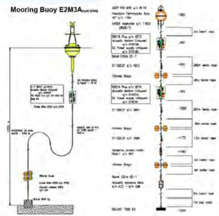
**Figure 2** – E2M3A configuration: surface buoy on the left (meteorological sensors + CT at 15m depth) and deep mooring scheme (CT, CTD and current-meters) on the right. The data presented in this work refer only to those collected by means of the deep mooring.
