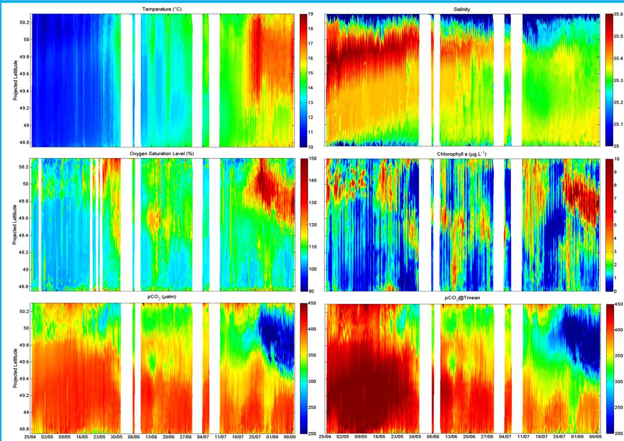
Figure 3. Surface distribution of temperature (°C), salinity, oxygen saturation level (DO%), Chl-*a* (µg L<sup>-1</sup>), pCO<sub>2</sub> (µatm) and pCO<sub>2</sub> normalized (µatm) at the mean temperature of 13°C (pCO<sub>2</sub>@Tmean) between Roscoff (48.7°N) and Plymouth (50.3°N) after sensors calibration.
