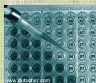
**Fig. 5:** Example of microplate where fluorescence is measured to determine the RNA / DNA ratio.
