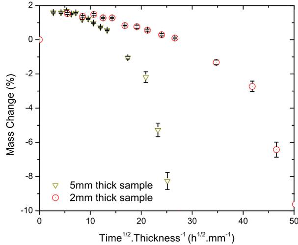
Figure 5: Mass change during ageing at 100°C in sea water
