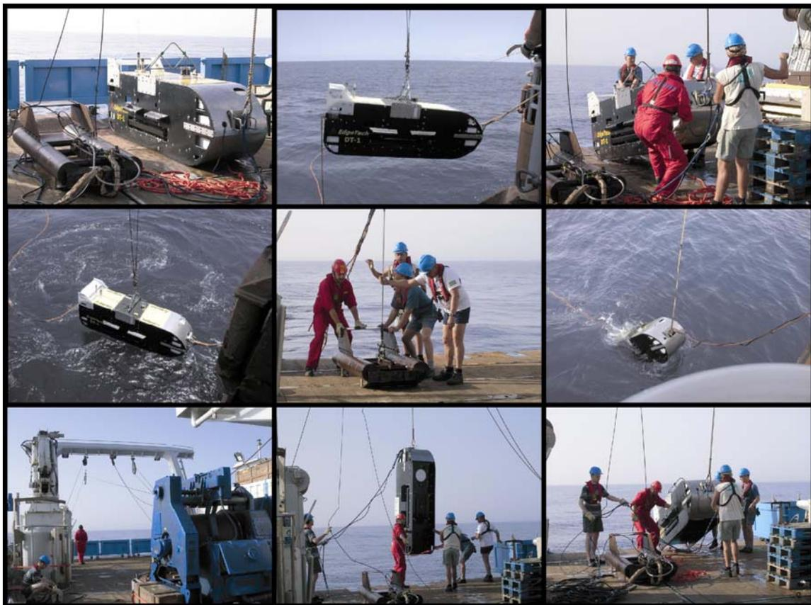
Figure 6.5 The DTS-1 towfish and the depressor weight during deployment and recovery (Courtesy of Klaucke and Foucher).
