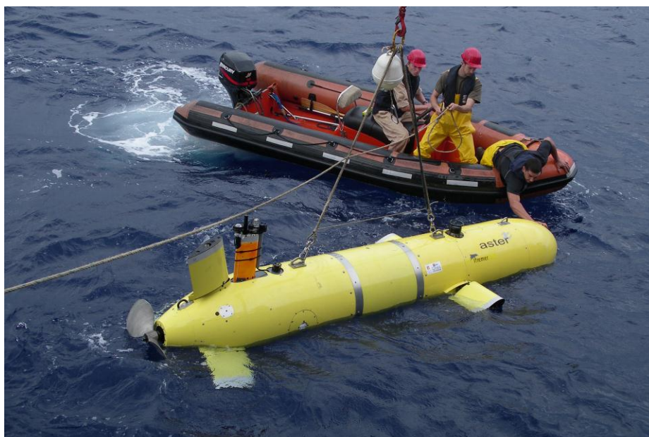
Recovery of the AUV after one of the Bionil dives.
