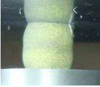
Figure 6. Barrelling effect on GSPU type 1 sample during uniaxial compression test
