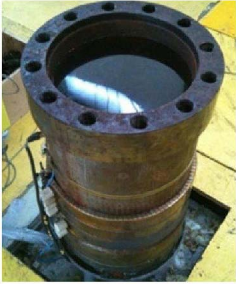
Figure 10. Photo of hydrostatic compression test system, internal diameter 300 mm
