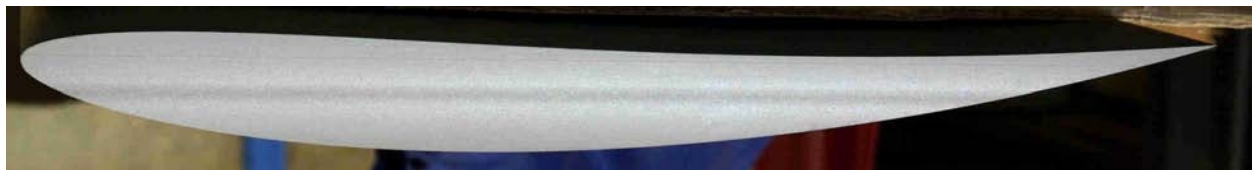
Fig. 3 NACA459 profile produced by numerical manufacturing.
