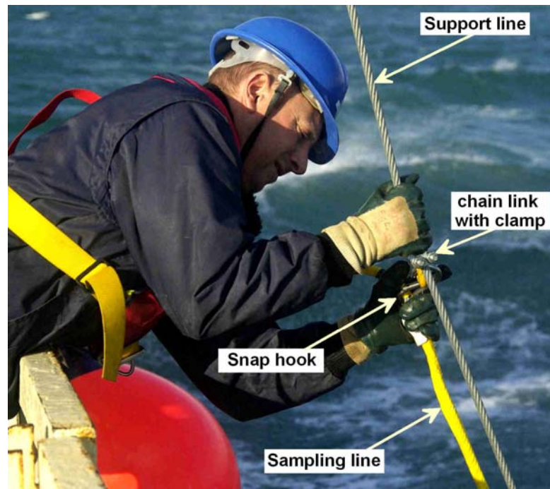
Fig. 2 Fixing the sampling line to the support line with snap hooks.
