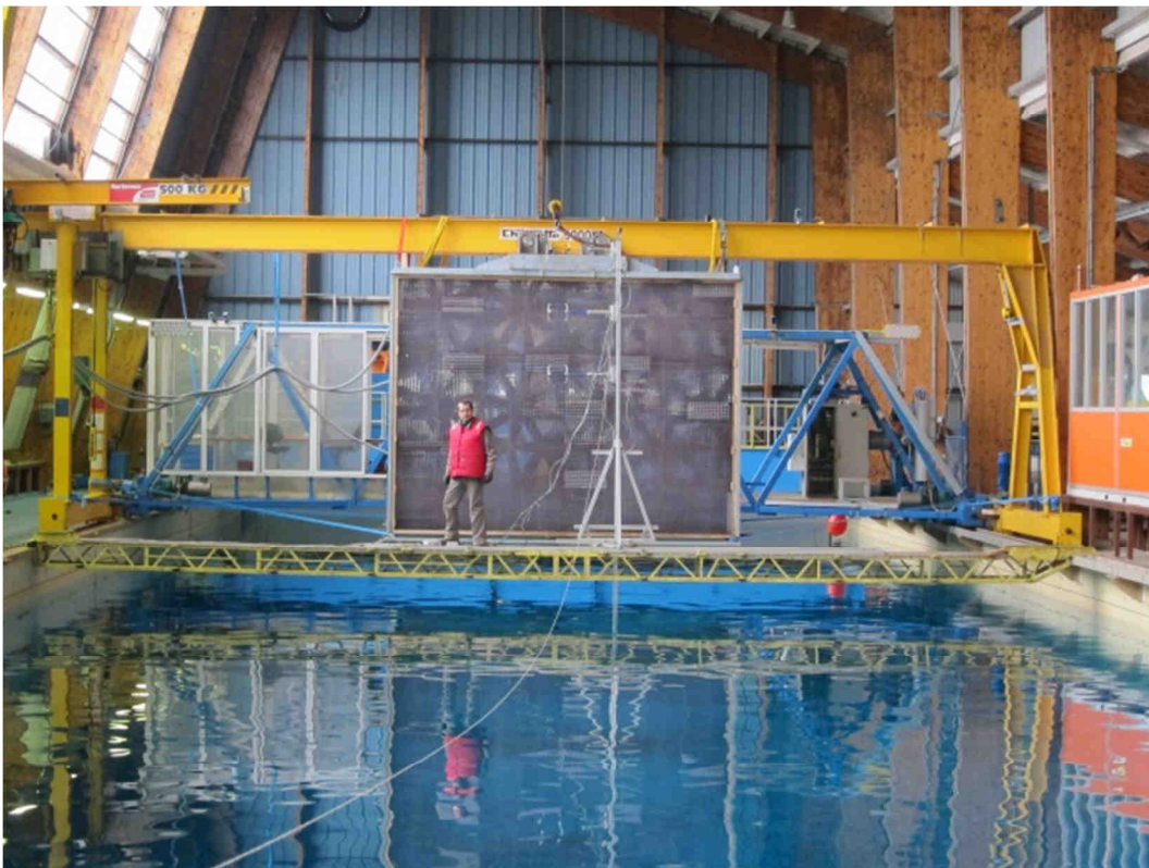
Figure 5.1: Wind generator at Ifremer wave basin
