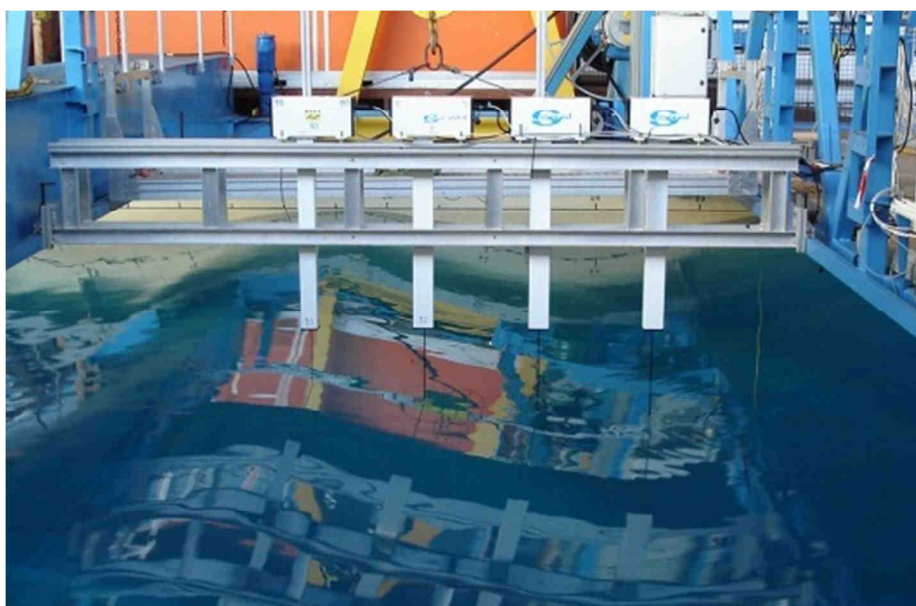
Figure 2.3: 4 wave gauges in a row measuring regular waves for wave characterization – Ifremer wave tank
