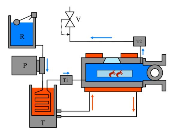
Figure S1. General schematic view of the BALIST aquarium. R : seawater reservoir ; P : high-pressure pump ; T : thermostat ; T1 and T2 : in-line temperature probes ; V : back-pressure valve. Arrows indicate the circulation of seawater (blue) or heating/ cooling fluid (red).
