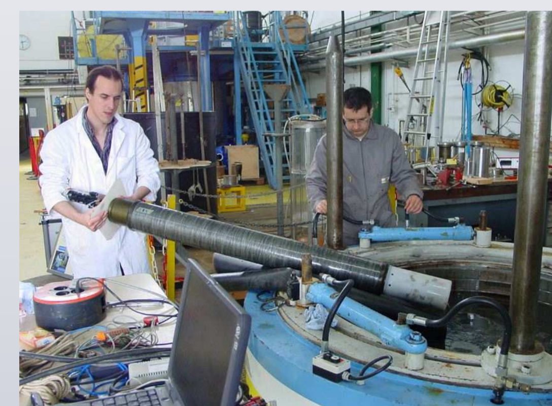
Pressure tank testing
