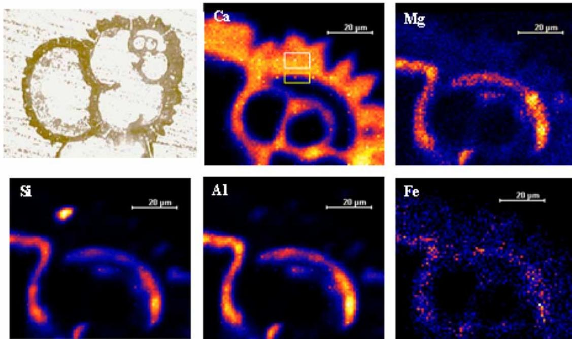
**Figure 2.** Example of element mapping. Areas analyzed are as follows: bulk shell material, white rectangle; coating, yellow rectangle. X-ray counts are represented for each element on an arbitrary color scale (brightness increases with X-ray counts).
