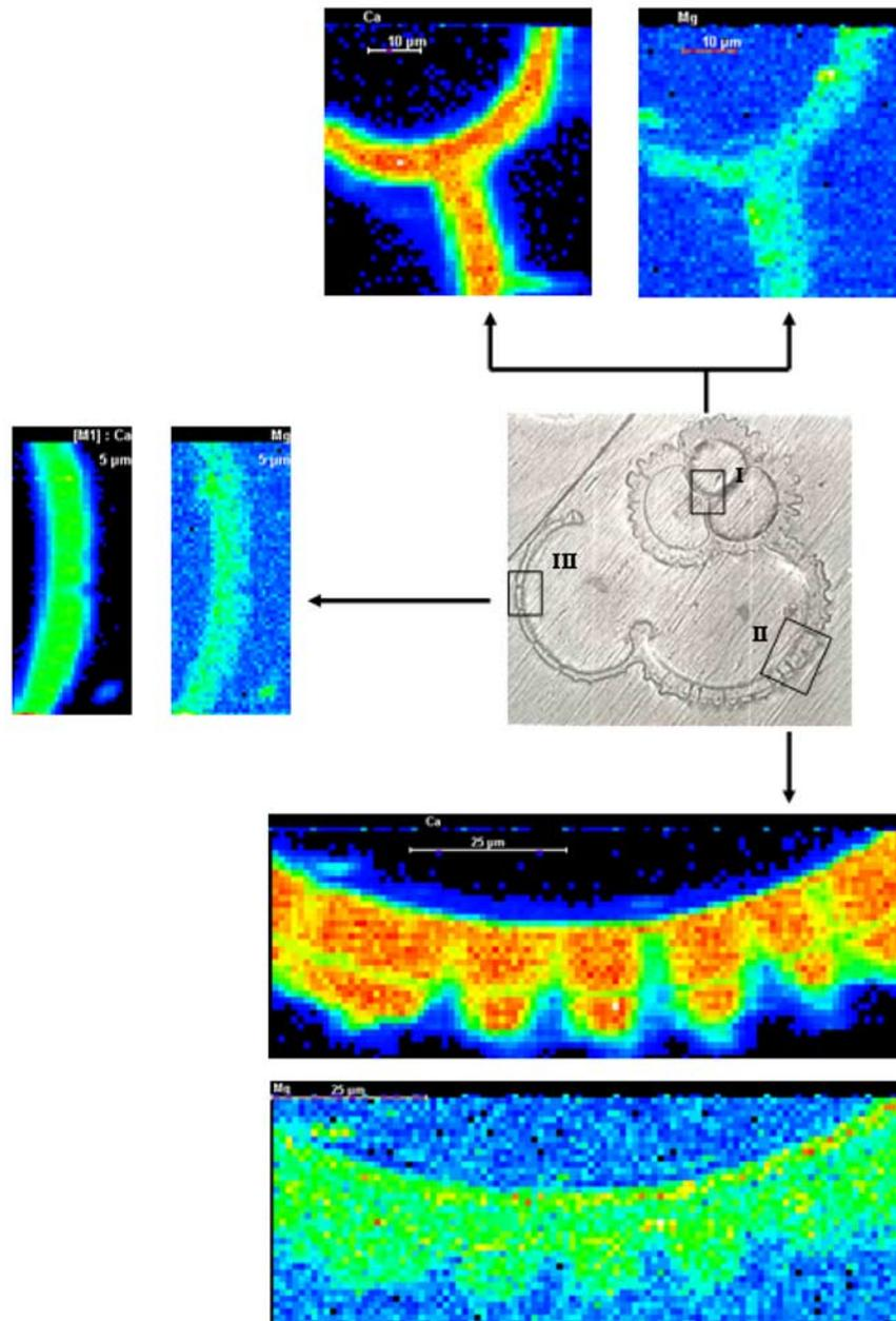
**Figure 3.** Regions identified for PIXE analysis on a single foraminifera shell (in this case the shell shown on Figure 1c). A distinction is made between early (I), intermediate (II) and final (III) chambers. The spatial distribution of Ca and Mg is shown for each of the three regions. X-ray counts are represented for each element on an arbitrary color scale (brightness increases with X-ray counts).
