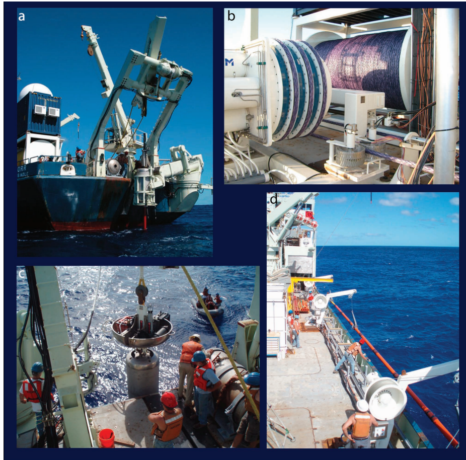
Fig. 1. The major components of R/V Knorr's new long core handling system: (a) stern view of the A-frame, boom sheave, and Lantec winch and stern-mounted grapple; (b) the traction winch and take-up drum for the Plasma rope; (c) the piston core head and release in vertical position, coupled and ready for lowering; and (d) the starboard davit cranes with a corer in horizontal position.
