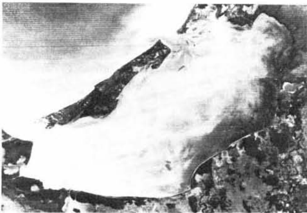
Figure 5 Landsat 2 image of Términos Lagoon, 16 January, 1978, during « nortes » season. Band 5, red for sediments and circulation. Photograph courtesy of Donald S. Graham (Tudor Engineering Company, San Francisco, California) and John M. Hill (Dept. Civil Engineering, Louisiana State University, Baton Rouge, Louisiana).
