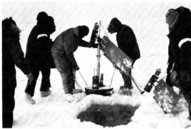
Figure 6 Deployment of current meters and tide gauge from fast ice in Stefansson Sound (SS) in November 1978.
