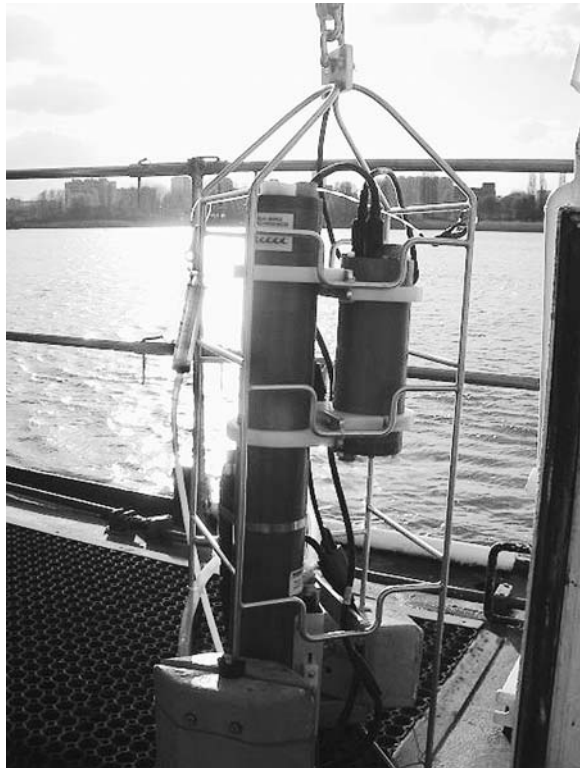
PLATE 1. A CTD (conductivity, temperature, and depth) probe, shown here at the Scheldt Estuary, was used at each site to measure the physical parameters of the water column. Photo credit: F. Gazeau.
