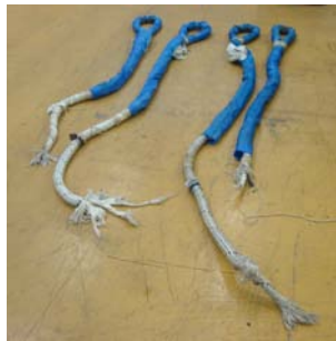
Figure 16: Failed rope samples ( left ) NS5 and ( right ) NS6 after load-to-failure tests LS4
