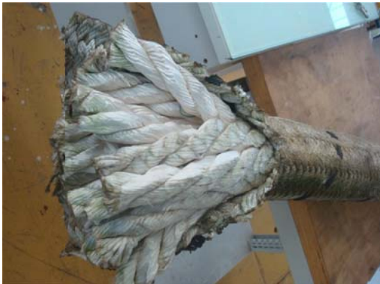
Figure 3. 400 ton break load parallel sub-rope construction. Braided jacket removed to show twisted 3-strand nylon sub-ropes.
