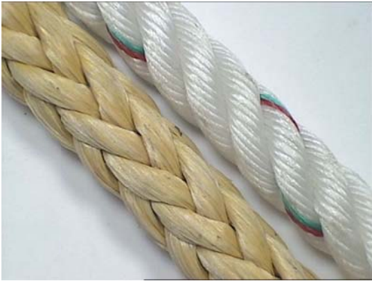
Figure 2. Examples of twisted and braided rope constructions
