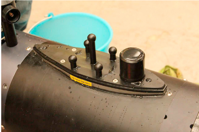
Fig. 3. The Underwater USBL Modem, installed at the SeaCat AUV.
