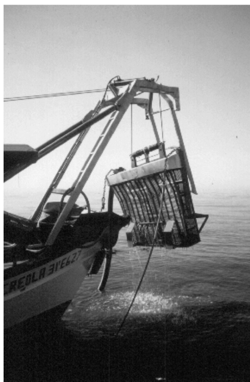
Figure 3-34. Hydraulic dredge for razor clams ( Ensis siliqua minor ) (by M. Pellizzato).
