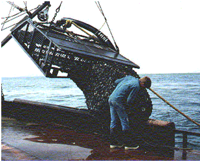
Figure 3-49. Hydraulic dredge filled with surf clams being hauled on board
