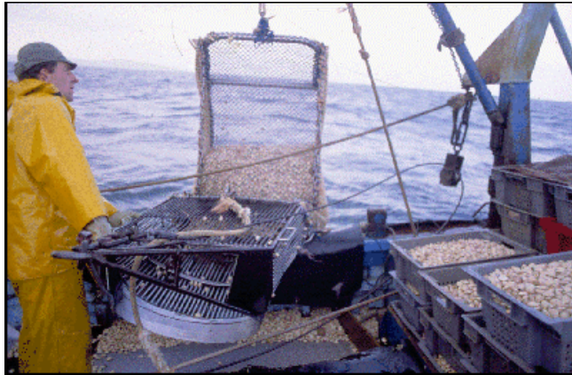
Figure 3-22. Thick trough shells dredge with short blade
