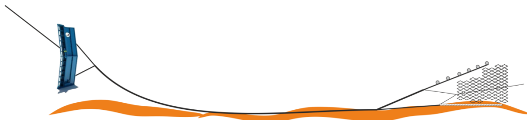
Figure 29. The use of flying/pelagic doors in bottom trawls
