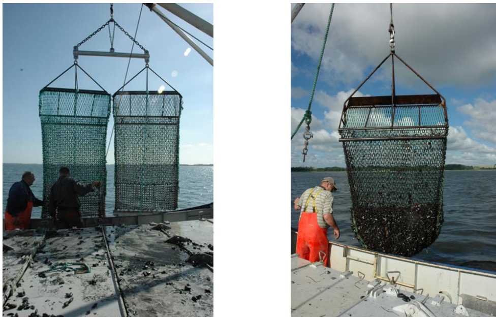
Figure 2. Different types of mussel dredges – light at the left and standard heavy at the right hand side.
