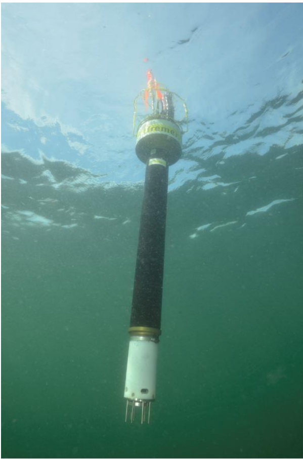
The Arvor-Cm profiling float in action (Photo courtesy of Olivier Dugornay, Ifremer)
