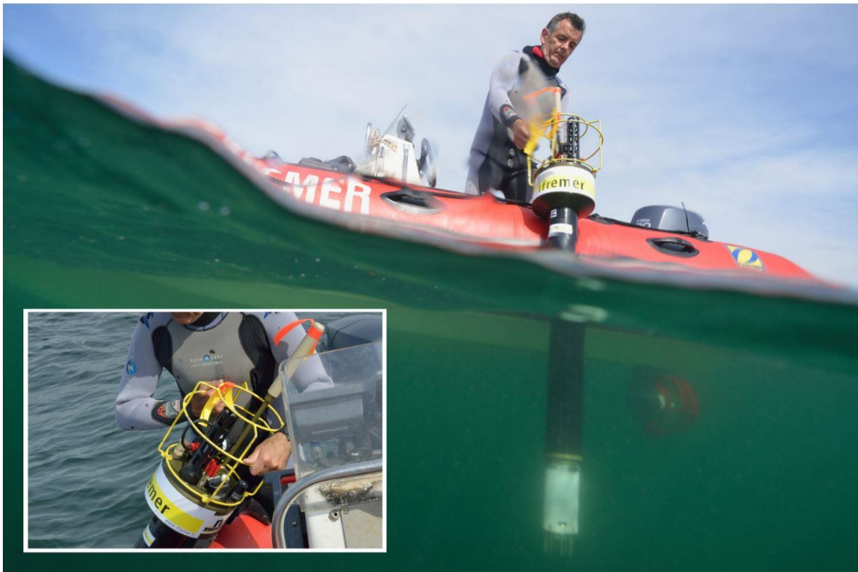
Arvor-Cm deployment in the Bay of Vilaine, France. (Inset) Close-up of the Arvor-Cm upper-end cap. (Photos courtesy of Olivier Dugornay, Ifremer)
