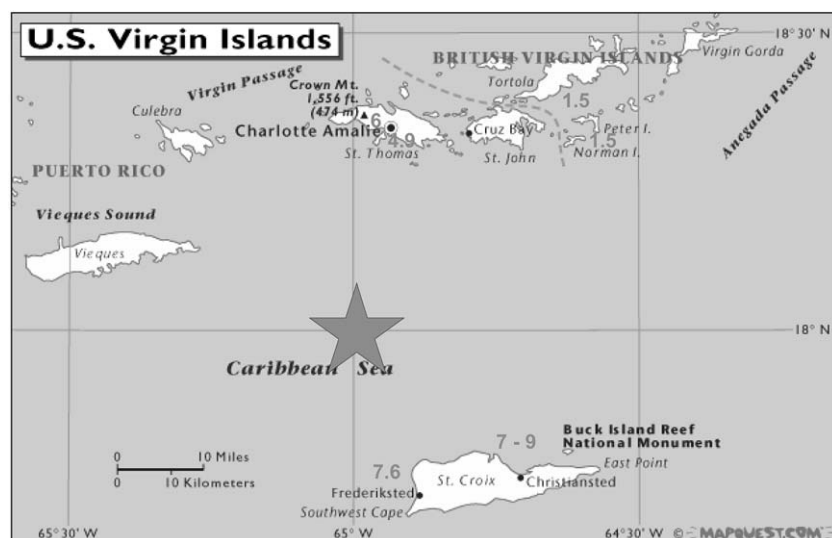
Fig. 1. The distribution of tsunami runup (meters) in the Virgin Islands (the epicentre is shown by star).
