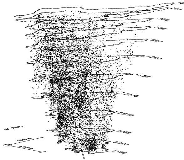
Figure 11. Three-dimensional view of particles' distribution after 5 years, with L = 4 km. Location of the release marked by R.
