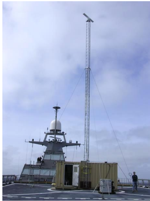
Fig. 2. Tower mounted X-Band (9410 MHz) wave radar temporarily installed on-board the U.S. Navy's FSF-1, Sea Fighter, to measure the wave field during sea trial.
