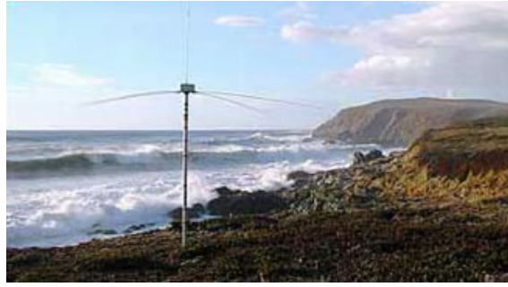
Fig. 3. - High frequency (HF) radar systems measure the speed and direction of ocean surface currents in near real time.
