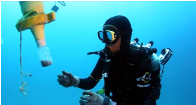
Figure 1. (a) Mesocosms ( \sim 50 \text{ m}^3 ) deployed in the framework of the VAHINE project. (b) Sediment traps screwed onto the base of the mesocosms and were sampled daily by SCUBA divers.
