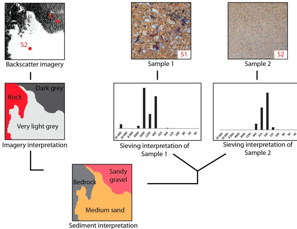
**Figure 1.** Methods for the creation of the sedimentological map of the Bay of Brest: in the left top corner the side-scan sonar (1:5000) analysis allowed us to define the backscatter variations (grey nuances); in the right top, sample analysis by the sieving method is translated into a histogram for each sieve and shows the final sedimentary interpretation.
