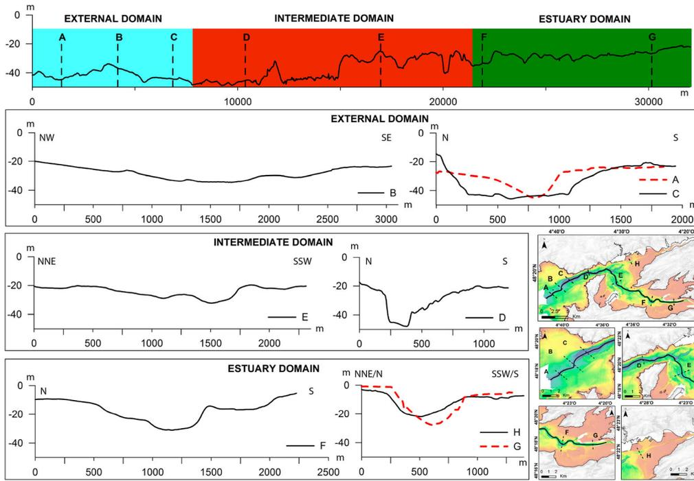
**Figure 2.** Shape of the paleo-footprints and their location on the maps on the right lower corner (scale of 1:90,000 and 1:30,000). On the top this is the profile that follows the channel from the Iroise Sea to the Aulne estuary divided in three main domains: external (blue), intermediate (red), estuary (green); shapes of each domain are illustrated.
