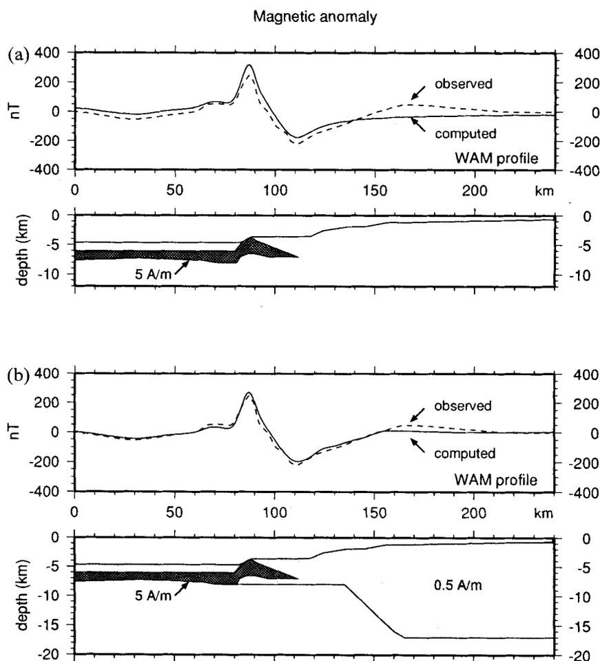
**Figure 3.** Forward modelling of magnetic anomalies along profile WAM, observed (dashed line) and computed (solid line). (a) a single magnetic body which represents the oceanic domain and the basaltic unit with a magnetization of  $5 \text{ A m}^{-1}$ , and (b) two magnetic bodies which represent the oceanic crust and basaltic unit with a magnetization of  $5 \text{ A m}^{-1}$  and the continental crust with a magnetization of  $0.5 \text{ A m}^{-1}$ .
