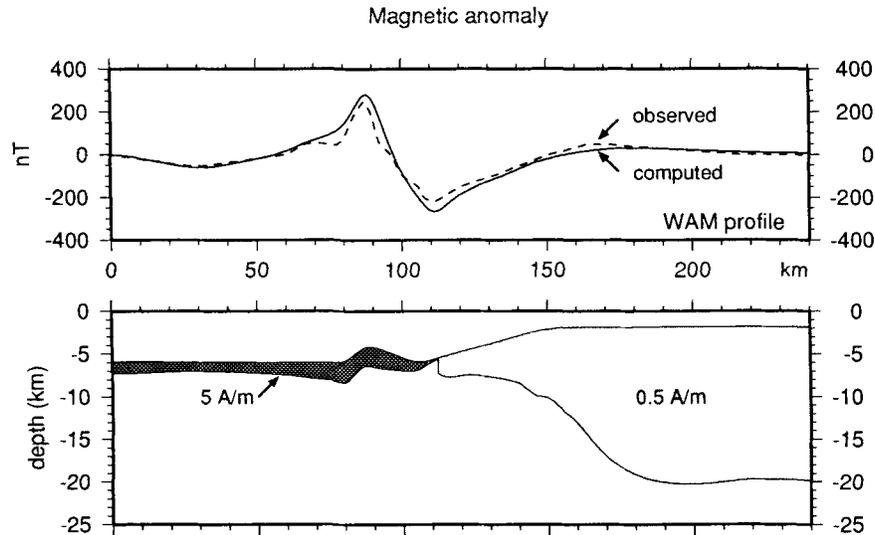
Figure 6. Composite model including results shown on Fig. 4(a) west of km 112 for the oceanic domain and on Fig. 4(b) east of km 112 for the continental domain. The resulting computed magnetic anomaly is in good agreement with the observed one.
