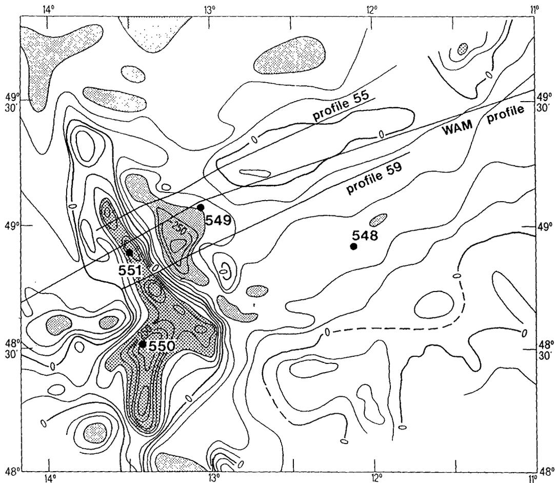
**Figure 2.** Magnetic-anomaly map of the Goban Spur area (Sibuet 1987) established from marine data. The contour interval is 50 nT. Dotted areas correspond to anomalies higher than 150 nT, fine dotted areas to anomalies lower than 150 nT. The horizontal extension of the volcanic sill located on the deepest tilted block is underlined by an elongated NW–SE anomaly.
