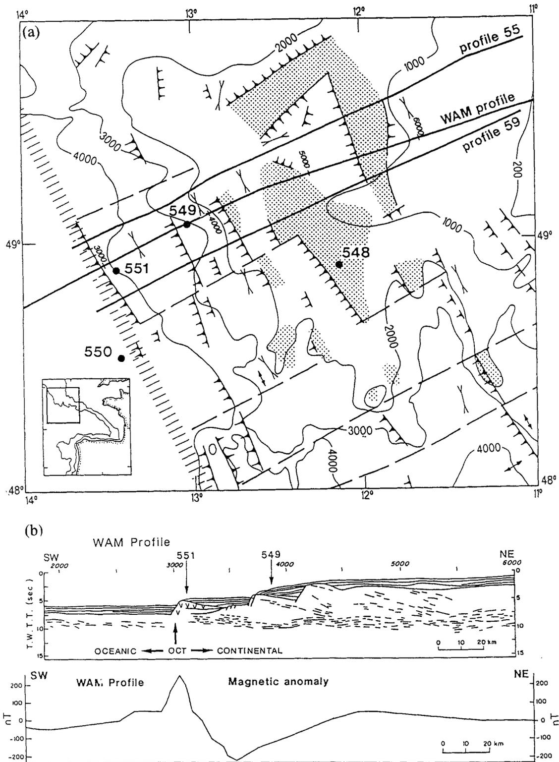
**Figure 1.** (a) Schematic structural map of the Goban Spur passive margin (Sibuet 1987) with the location of profiles WAM and Norestlante 55 and 59. DSDP sites 548–551 are denoted by black dots; long-dashed lines: transverse faults; lines with orthogonal ticks: normal faults; dotted pattern: lower Cretaceous eroded surfaces; dashed pattern: ocean–continent transition. (b) Line drawing of profile WAM and associated magnetic anomaly.
