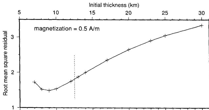
**Figure 5.** Root-mean-square residual between observed and computed magnetic anomalies versus the initial depth assuming a magnetization of  $0.5 \text{ A m}^{-1}$ . For initial thicknesses smaller than  $12 \text{ km}$  (vertical dotted line), the inversion process leads to negative thicknesses and its results are therefore discarded.
