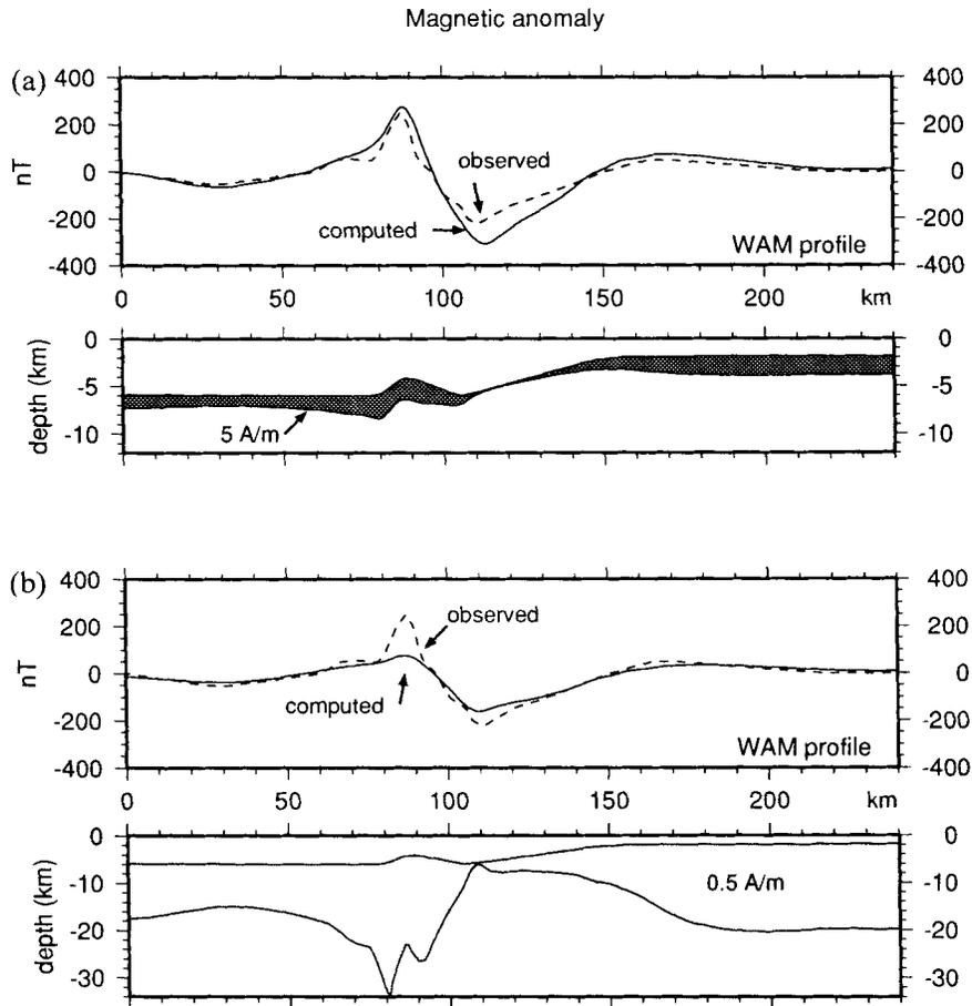
**Figure 4.** Inversion of magnetic anomalies along profile WAM. Top: observed (dashed line) and computed (solid line) magnetic anomalies. Bottom: magnetic body obtained by inversion assuming (a) a magnetization of  $5 \text{ A m}^{-1}$  and an initial thickness of the oceanic magnetic layer of  $1.5 \text{ km}$ ; (b) a magnetization of  $0.5 \text{ A m}^{-1}$  and an initial thickness of  $13 \text{ km}$ .
