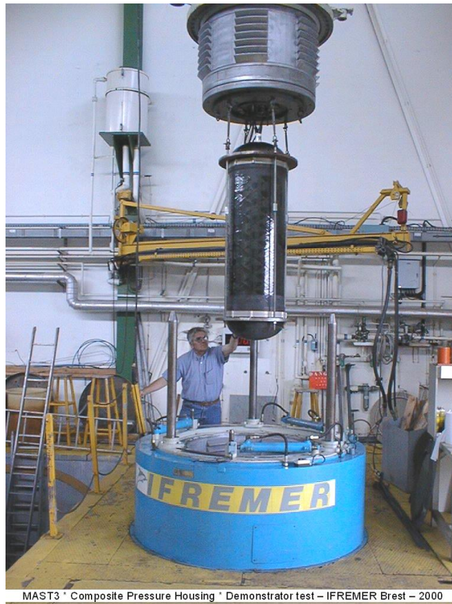
FIGURE 5: 40MM THICK COMPOSITE CYLINDER BEFORE IMPLOSION TEST.
