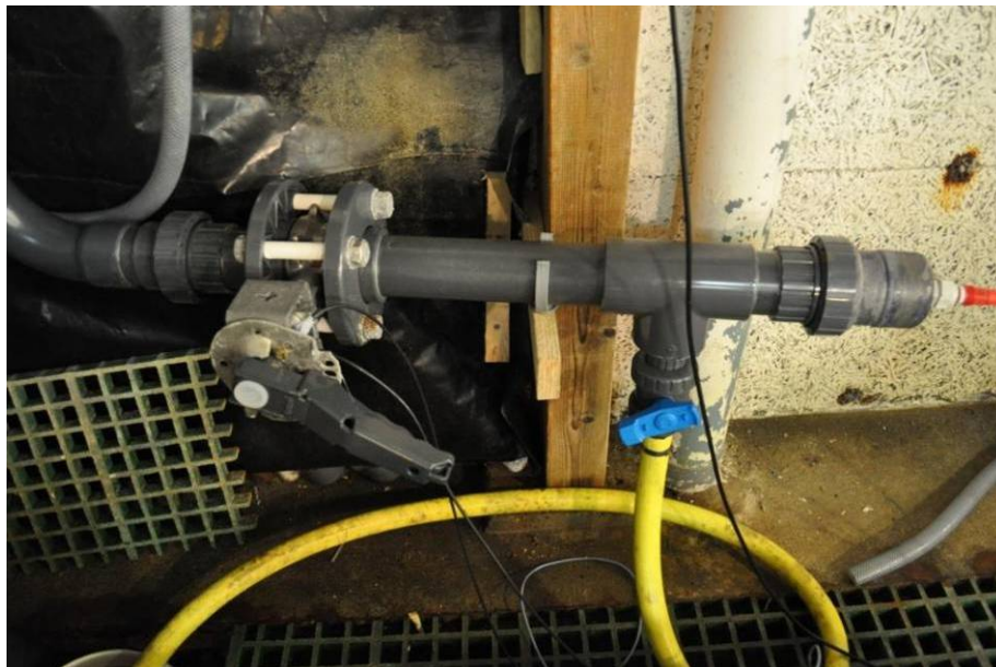
Figure 5: Photograph of the 316L butterfly valve in the set-up
