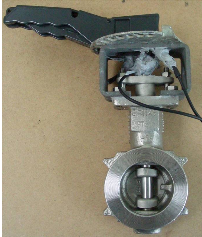
Figure 4: Photograph of the 316L butterfly valve before exposure
