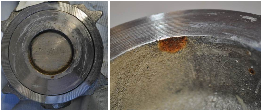
Figure 10: Photographs of butterfly valve after one month at impressed potential of -400 mV/SCE
