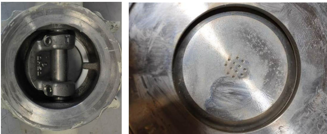
Figure 11: Photographs of butterfly valve after one month at impressed potential of -600 mV/SCE
